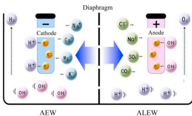
**Figure 1.** Generation of AEW and ALEW in an electrolytic cell, consisting of anode and cathode connected through an external power supply and separated by a septum or diaphragm.<sup>2</sup>
